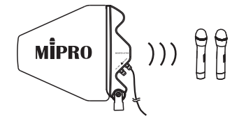
(Figure 4: × Wrong setup)
