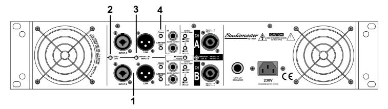
1. There are two **INPUT CONNECTORS** per channel. One is a combination 3 pin XLR and 3 pole (TRS) ¼" jack socket, the other a male XLR for linking to other amplifiers. Both balanced and unbalanced signals can be used to drive the amplifier.
