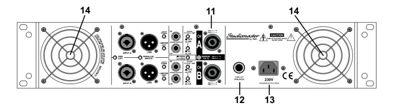
11. **Speaker Wiring**. Each channel uses SPEAKON NL4 connectors. Using cable as specified (See CABLES) speaker connections are as follows:-
